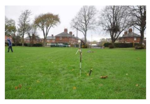
Two Abney levels were used in these tests and each operator carried out the test with both Abney levels. Each trekking pole was observed from the other with the Abney level supported on the top of the pole. (Earlier this day the calibrations of the two Abney levels had been checked with a variation of the "Two Peg Test" which was described in Section 5). Neither operator with either Abney level could discern any height difference between the two trekking poles when viewed from both directions.
