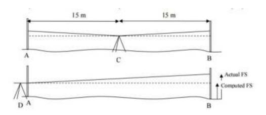
Now the problem with this method is that the average Abney level user may not have access to two surveyors' staffs and a tripod. Also it would be very difficult (impossible?) to make an accurate staff reading with an Abney level at a distance of 30m. So is there a simpler method that incorporates the principles of the "Two Peg Test"? The answer is "Yes" and an assistant is needed to do it.
