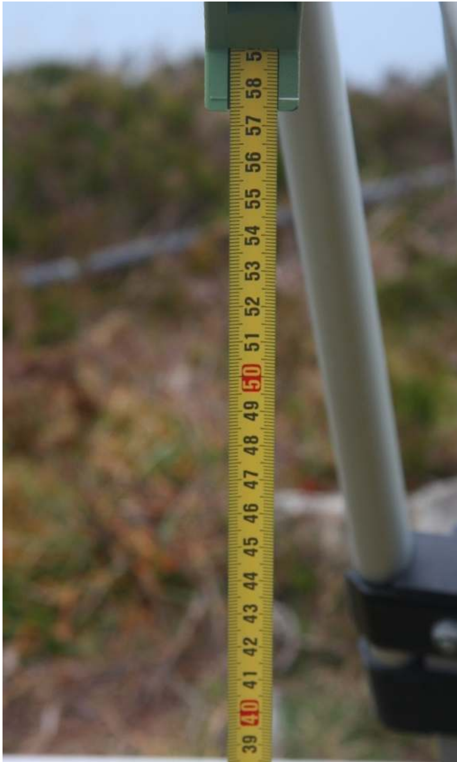
Viva GS15 setup showing 0.577m vertical offset
