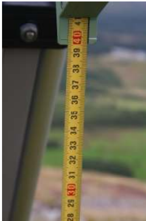
Viva GS15 setup showing 0.399m vertical offset
