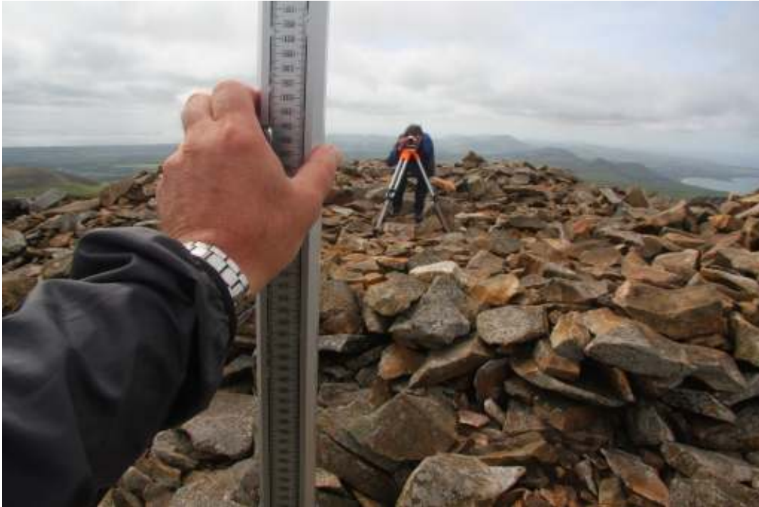
Surveying for summit position; G Jackson with Leica NA730
