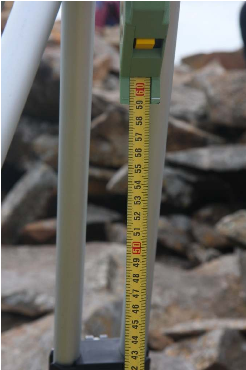
Viva GS15 setup on short tripod showing 0.594m vertical offset
