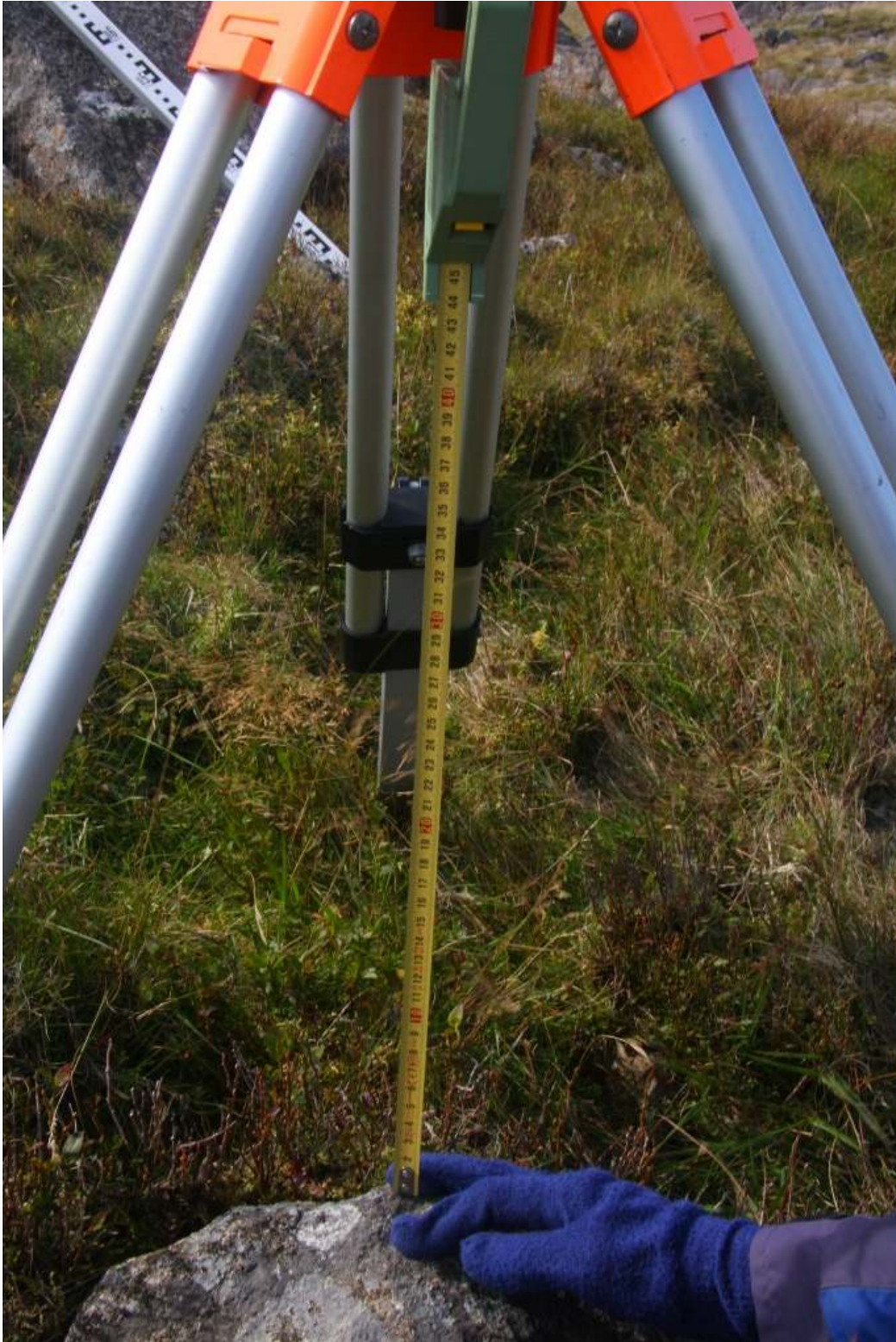
GS15 setup position on short tripod showing 0.443m vertical offset
