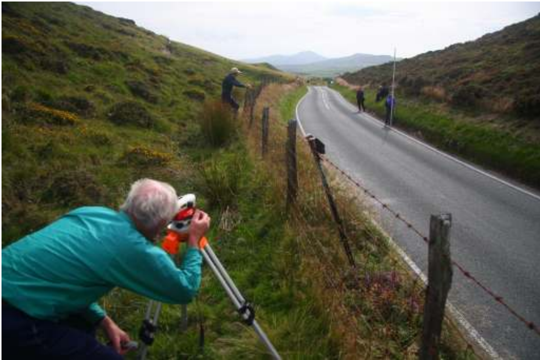
Survey for Bwlch position: J Barnard at Leica NA730
